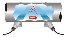
An ultrasonic meter equipped with heat flow capabilities measures the rate and quantity of heat delivered or removed from devices such as heat exchangers. By measuring the volumetric flow rate of the heat exchanger liquid, the temperature at the inlet pipe and the temperature at the outlet pipe, the energy usage can be calculated.
